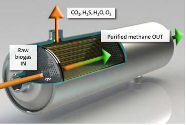
PRISM membrane separators for biogas upgrading contain thousands of tiny hollow fibers. Smaller gas molecules, like carbon dioxide and water vapor, diffuse through the membrane walls while the larger methane molecules are transported the length of the tube and exit from the end of the module.
