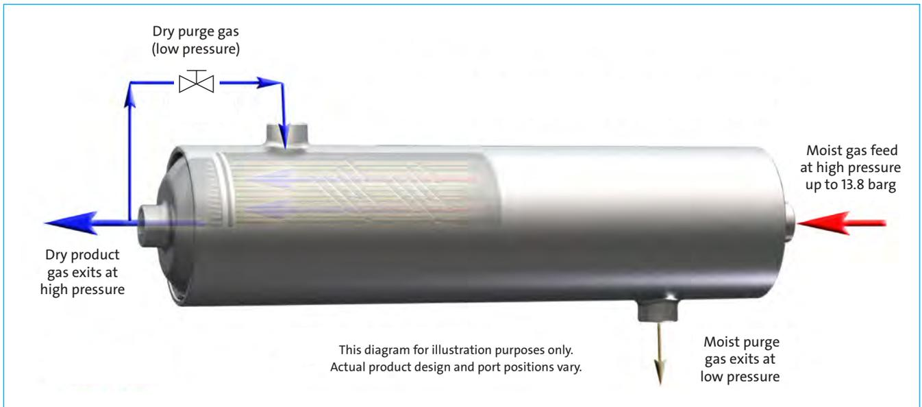
**Membrane dryers passively produce dry air with no moving parts or electrical components, consumable items, or desiccant dust carry-over. They provide silent and uninterrupted operation for a wide range of dew point specifications.**
