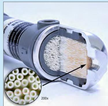
A typical membrane separator contains thousands of fibers that are bundled and encased at both ends in epoxy resin. The ends of the bundle are cut, which leaves the fiber bores open on both ends, allowing the gas to travel from one end to the other. The fiber bundle is enclosed in a suitable casing. The casing protects the fibers and routes the gas properly.
