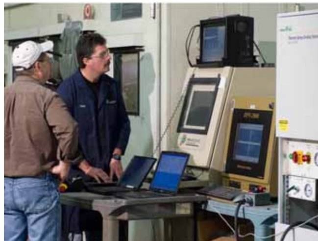
With our thermal spray cooling technology's advanced system, you can monitor your spray operation from the control room. The temperature profile for your operation will be displayed on your computer screen and captured for future analysis, playback and audits.
