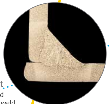
Ferromaxx® 7 MAG fillet weld in 3mm thick BS970:080M50 steel
