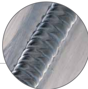
TIG butt weld in 10mm thick 4140 aluminium alloy using Alumaxx® Plus
