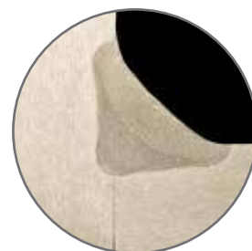
MIG fillet weld in 10mm thick 4140 aluminium alloy using Alumaxx® Plus
