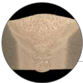
Ferromaxx® 15 MAG butt weld in 12mm thick BS970:080M50 steel
